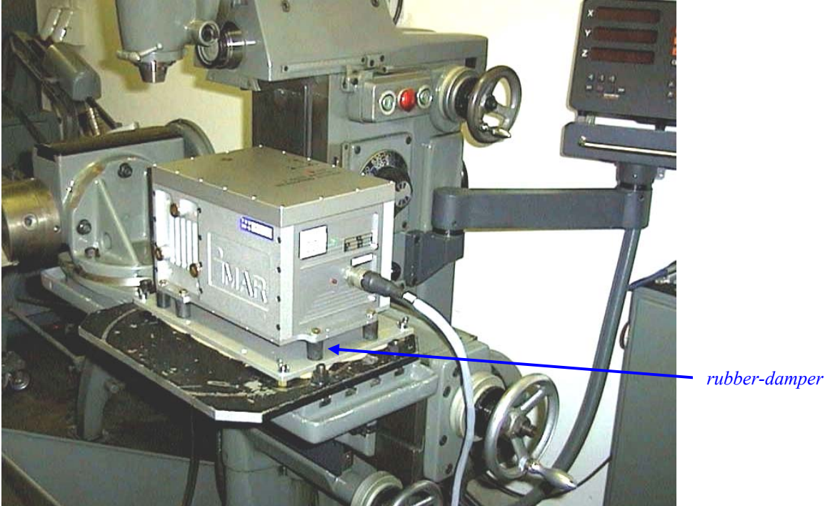
Fig. C-1 IMU's mount using rubber-damper
