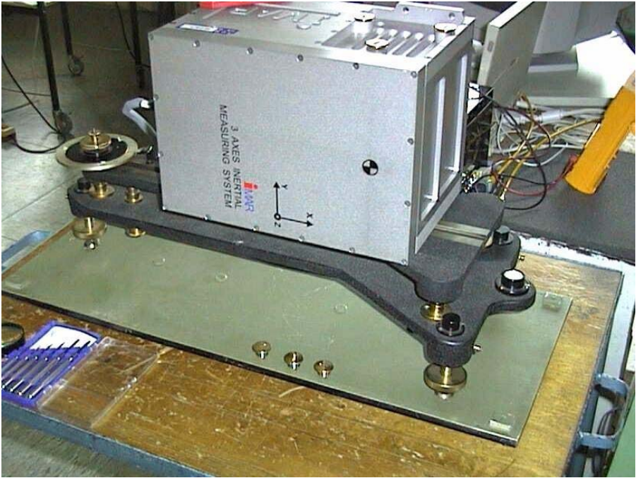
Fig. B-2 Rotated IMU on the tilting-table (y-axis upwards)
