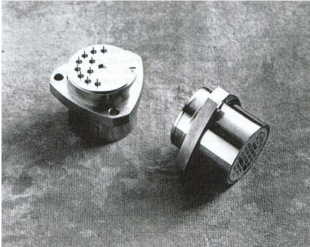
Fig. A-1 QA2000 Honeywell balancing accelerometer: external view
