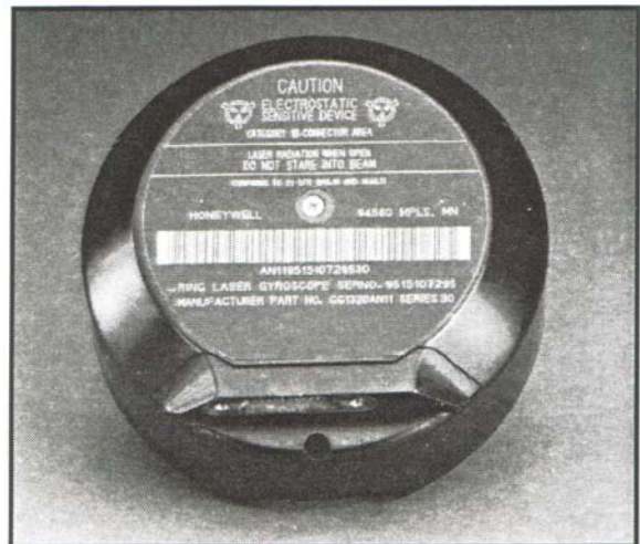
Fig. A-4 GG1320 Honeywell Ring Laser Gyroscope: external view
