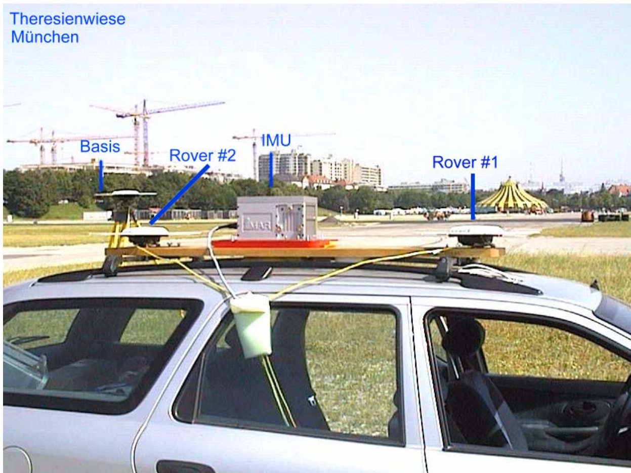
Fig. 1 DGPS/INS car-experiment in Munich
