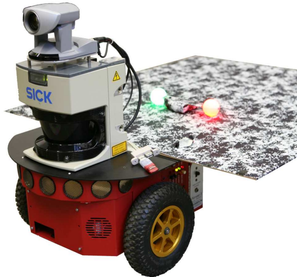
Fig. B.1: The Pioneer P3-DX mobile robot with two active markers.
