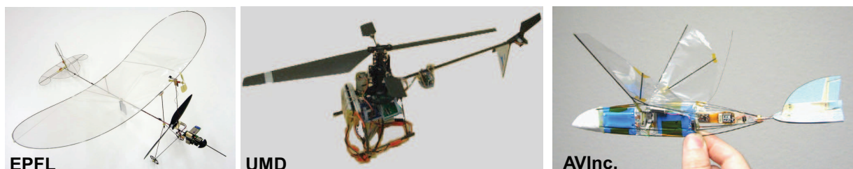
Fig. 2.1: Various MAV platforms. Left: a fixed-wing MAV – the microflyer from EPFL [130]; middle: a rotary-wing MAV from UMD [59]; right: a flapping-wing MAV – the Microbat from AeroVironment [77].
