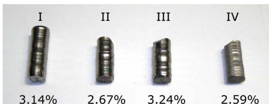
Figure 5.2.1: Photo of the four \text{Pd}_{1-x}\text{Ni}_x crystals from Mateck grown by the Czochralski technique. These samples have a cylindrical shape with a diameter of \approx 10\text{mm} and lengths between 26 mm and 35 mm. The crystals will in the following be referenced by their numbers I to IV.
