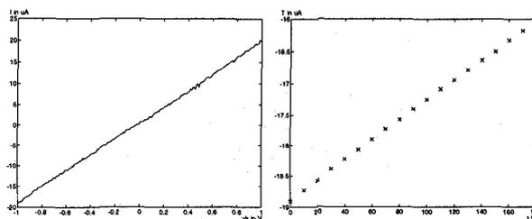
Figure 5: (a) Dc transfer characteristic of the analog memory and (b) measurement of the storage time.
