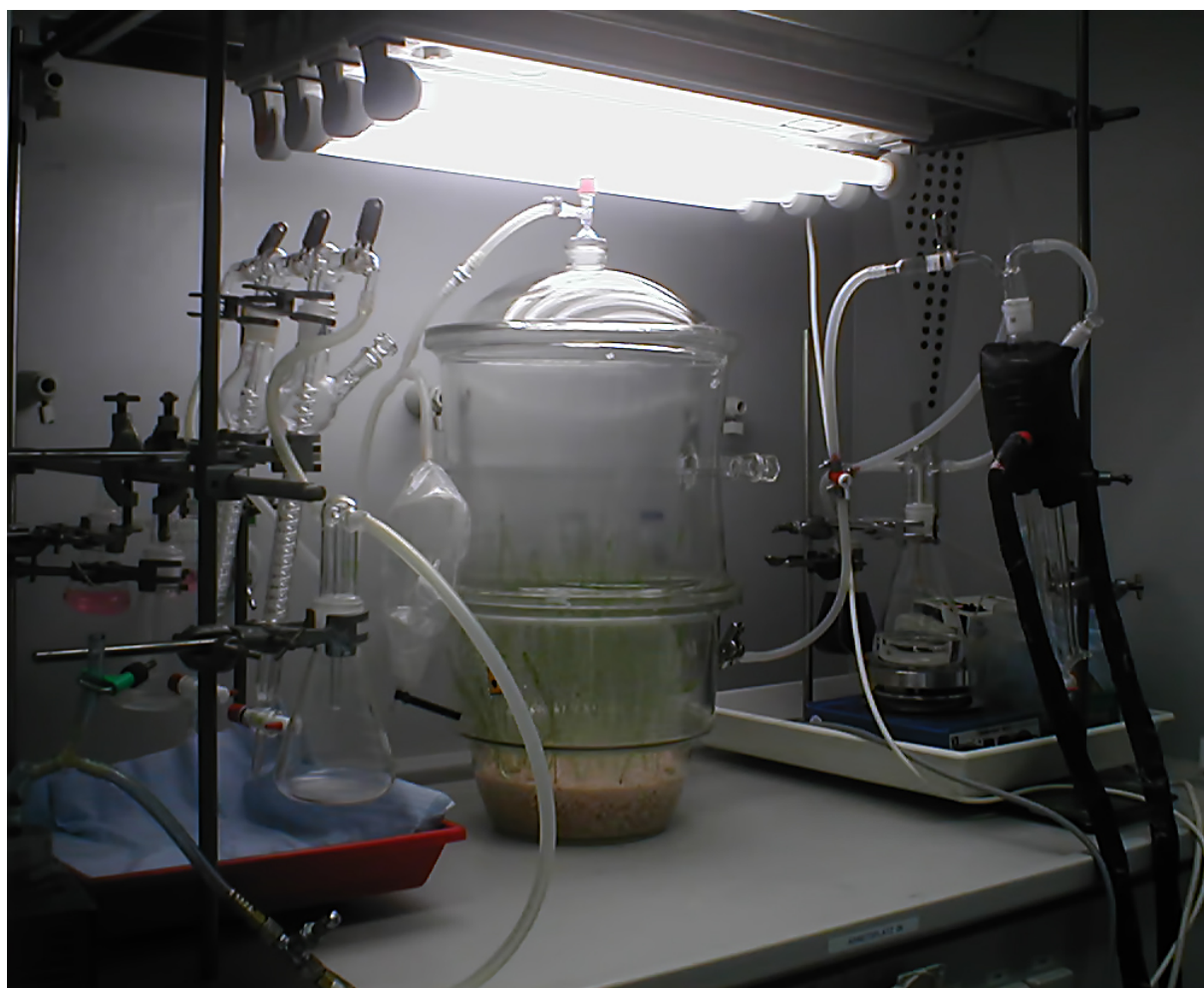
Figure C.1: Photograph depicting experimental setup for ^{14}\text{C} labeling of barley plants. The barley plants were grown in a desiccator under a light source (section 2.2). ^{14}\text{C} labeled \text{CO}_2 was produced continuously by dripping ^{14}\text{C} -carbonate into hot concentrated phosphoric acid.
