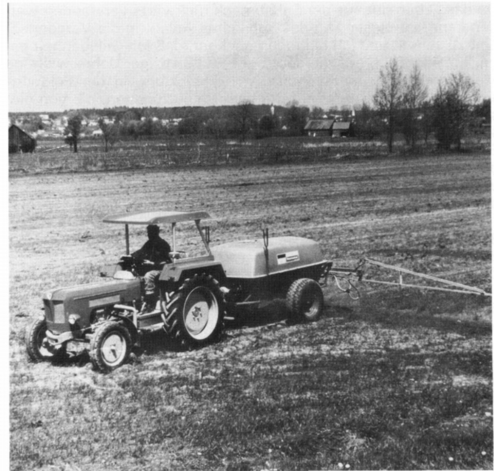
Abb. 2: Der "kleine", 35 PS-starke Schlüter-Schlepper Super 350
