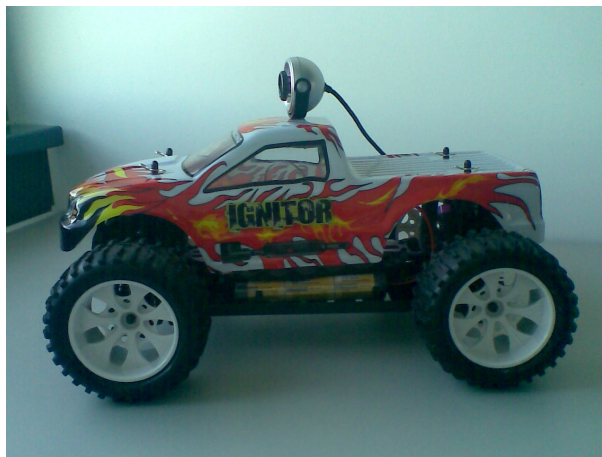
Figure 8.4.: The CamCar with the USB webcam on the roof
