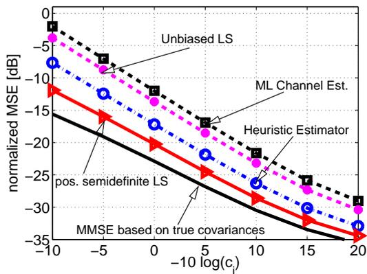
Figure 5. Normalized MSE of MMSE channel estimator (6) for different estimators of  $C_h$  and  $C_{n,S}$  compared to ML channel estimation (Scenario 2,  $B = 100$ ).
