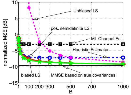
Figure 2. Normalized MSE of MMSE channel estimator (6) for different estimators of  $C_h$  and  $c_n$  compared to ML channel estimation (Scenario 1,  $c_n = 1$ ).
