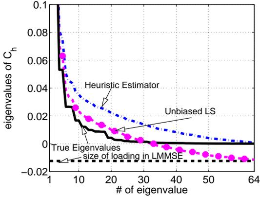
Figure 1. Eigenvalues  $\lambda_i/\lambda_1$  of true channel covariance matrix  $C_h$  and different estimates  $\hat{C}_h$  ( $B = 100$ ). Solid horizontal line shows negative value of loading, i.e.,  $-\hat{c}_n^{LS}/(N\lambda_1)$  (cf. Eq. 7), in the MMSE estimator to illustrate problem of ill-conditioned inverse in (6).
