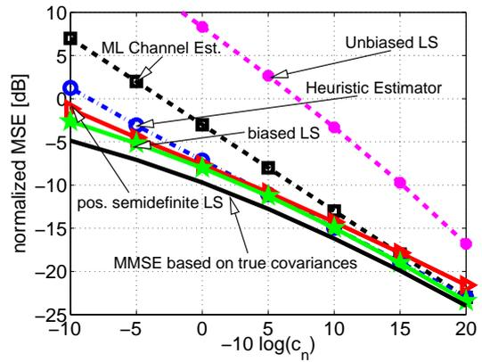
Figure 3. Normalized MSE of MMSE channel estimator (6) for different estimators of  $C_h$  and  $c_n$  compared to ML channel estimation (Scenario 1,  $B = 100$ ).
