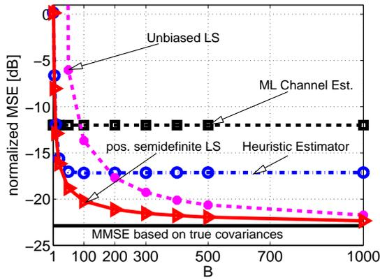
Figure 4. Normalized MSE of MMSE channel estimator (6) for different estimators of  $C_h$  and  $C_{n,S}$  compared to ML channel estimation (Scenario 2,  $c_1 = 1$ ).
