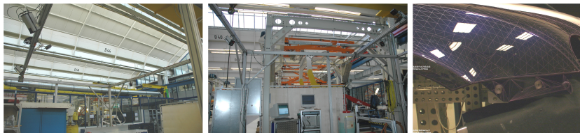
Fig. 8.1. Tracking setup with four cameras in an industrial environment (left, middle). Virtual overlay on a real car part (right).
