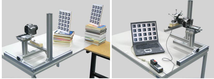
Fig. 7.15. Setup for the DRC Off-Line Phase: Calibration of the intrinsic camera parameters (left) and calibration of the display plane by taking several pictures with the HMD at a fixed position and the camera moved horizontally (right).
