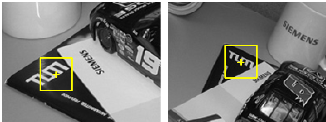
Figure 5.3: The classic 'corner + fixed window' strategy for finding correspondences is not suited for wide-baseline conditions.
