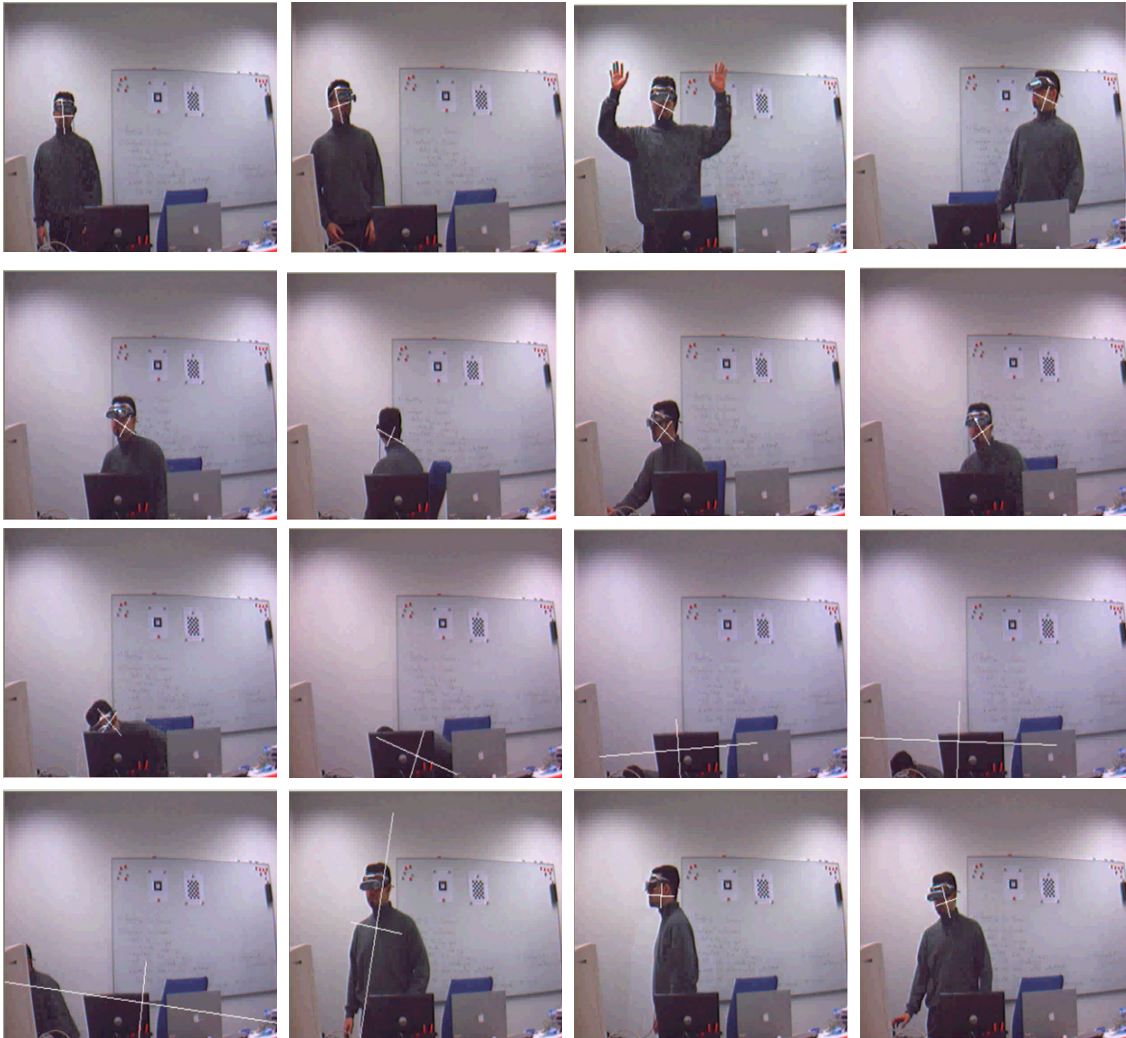
Figure 4.9: Real time face tracking system based on the Continuously Adaptive Mean Shift (CAMSHIFT) algorithm [18]. The two perpendicular white lines are the two main axis of the error ellipse in the image.
