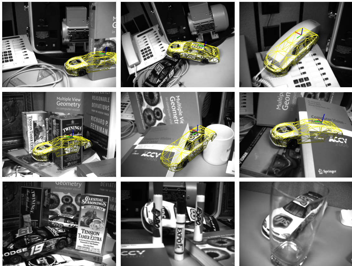
Figure 7.4: Detection results of the toy car. The last row show some cases where detection fails due to large occlusions combined with cluttered background or large distortions of the texture structure e.g. when seen from behind a convex glass.
