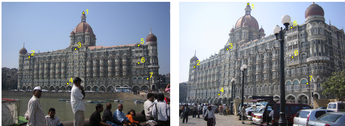
Figure 5.1: Two images from different views of the same scene (Taj Mahal Hotel, Mumbai (Bombay), India). Feature points with the same number correspond.
