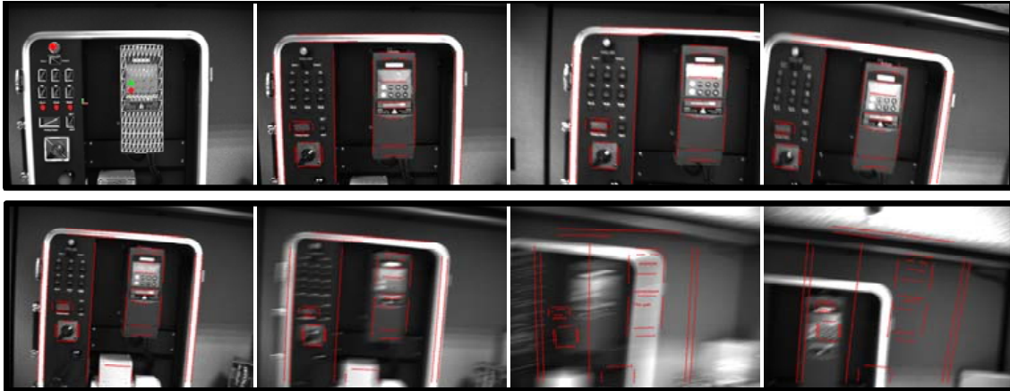
Figure 1.3: The initialization problem. Each time tracking is lost, e.g. due to fast camera motion causing blurred images, the tracking system needs to be initialized again.
