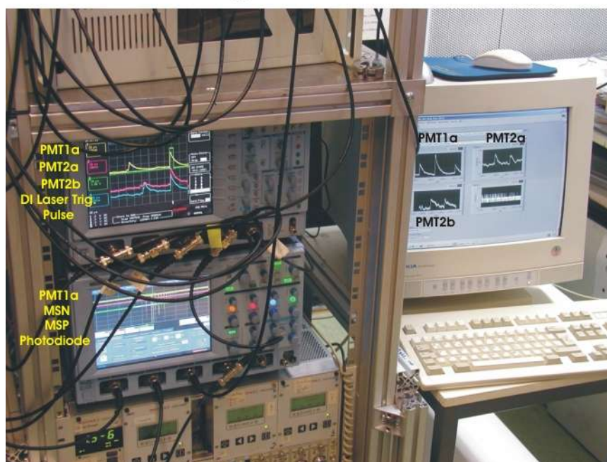
Figure. 50 : Setup of the SPALMS data acquisition unit ( scheme Nr.1)
