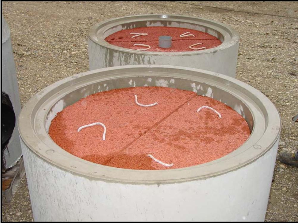
**Figure 25:** The porous concrete barrier material (HydroCon).
