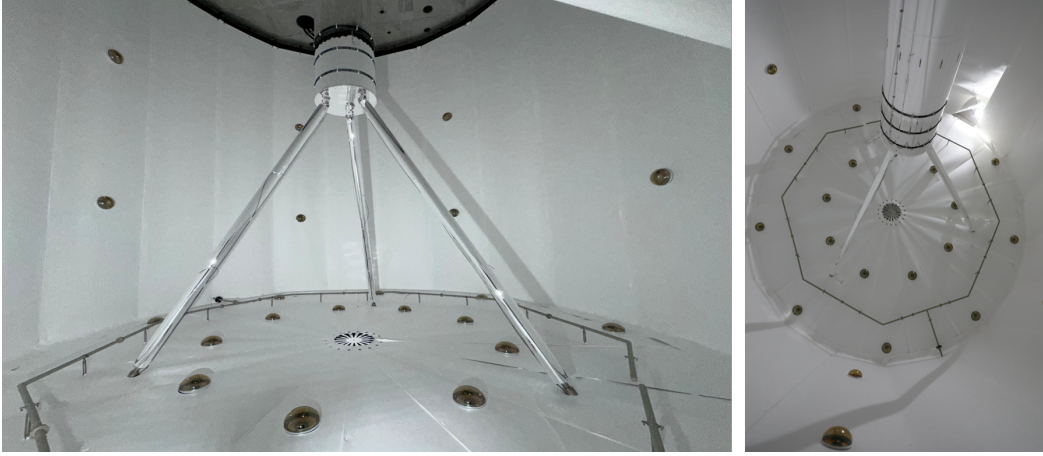
Figure 3.14: Muon veto within the water tank. The walls and floor are covered in a reflecting Tyvek foil. The drywell, and the tripod it connects to, are covered in specular reflecting foils. In total, 30 PMTs are distributed over the tank mantle and bottom.
