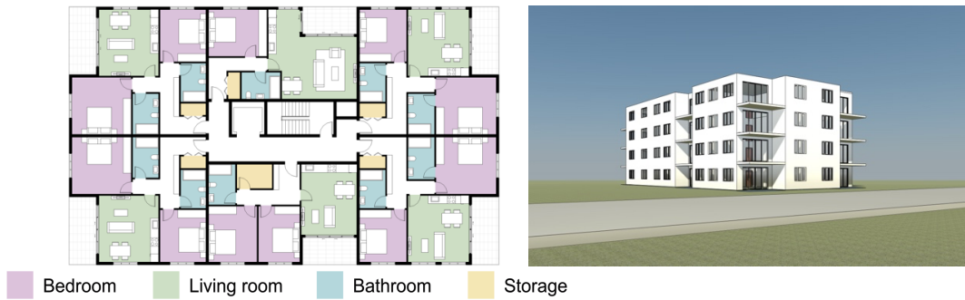
Figure 7: Typical floor plan formed with the plan selected in Figure 6 (left) Figure 8: A basic form of the entire building formed from the typical floor plan (right)
