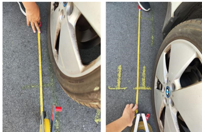
Figure 11. Stop position accuracy measurement.
