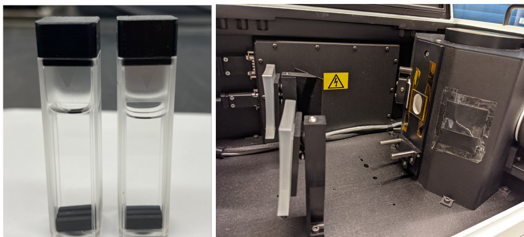
Figure 13. Left: PEN pieces inserted into cuvette (on left) and reference cuvette (on right) without samples. Slotted black pieces were used in both the sample cuvette and the reference cuvette to ensure consistency. The cuvettes are then placed in a Shimadzu UV-2700i UV-Vis Spectrophotometer. Right: inside of UV-VIS Lambda 850 spectrometer in transmission mode. A PEN sample was placed at the opening of an integrated sphere.
