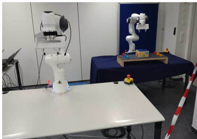
Figure 19: Photo of the experiment setup. The leader arm (left) has no controller currently installed
