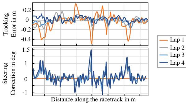
**FIGURE 9.** Qualitative demonstration of a learning-based control approach based on [101]. For each new lap the car is decreasing the tracking error by applying a higher correction steering angle for each vehicle movement.
