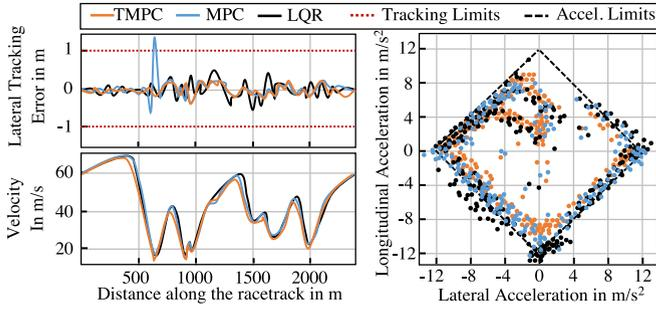
**FIGURE 8.** Qualitative comparison of an LQR, MPC and Tube MPC controller in an autonomous racing setup based on [216]. While the MPC is outperforming the LQR controller, it can be seen the Tube-MPC is not violating any dynamical constraints, e.g., the maximum lateral and longitudinal acceleration.
