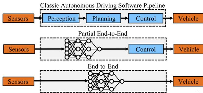
**FIGURE 10.** Classic autonomous driving software pipeline in comparison to partial and full end-to-end software pipeline.
