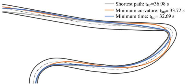
**FIGURE 5.** Comparison of global optimal raceline algorithms based on shortest path, minimum-curvature [78] and minimum-time [43] optimization, which lead to different lap times  $t_{lap}$  and trajectories.
