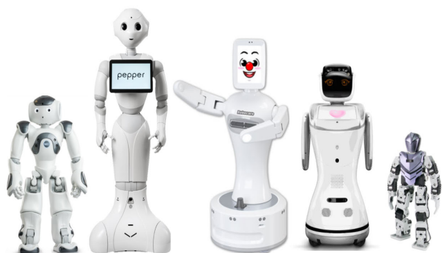
FIGURE 4. Humanoid Robots applied in ADHD treatments. From left: NAO, Pepper, Silbot, Sanbot Elf, and Bioid.
