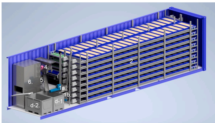
Fig. 2. Cutaway overview of the H. illucens rearing module. Devices are classified as follows: 1a. shredder, 1b. screw feeder, 2. reactor, 4. sieve, 5. blancher, 6. dryer, d-1 frass storage, d-2 dried insects' storage.
