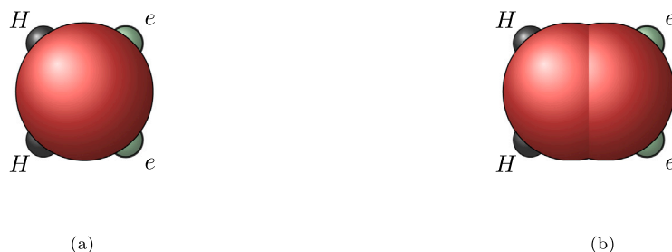
Fig. 5. Schematic for two possible SAFT models for water. The molecule is represented by a number of spherical segments ( m ), which interact via a potential (in SAFT-VR this is the Mie potential) with a repulsive core diameter \sigma . The Mie potential is characterized by a repulsive exponent ( \lambda^r ), an attractive exponent ( \lambda^a ), and a well depth \epsilon . These segments are indicated by the spheres shaded red. In (a) the molecule is assumed to be spherical with just one segment ( m = 1 ). In (b) the molecule is non-spherical and 1 < m < 2 , represented by two fused spheres. In (a) and (b) the hydrogen bonding is represented by a 4-site association scheme (2 e sites and 2 H sites), corresponding to the two lone pairs of electrons on the oxygen atom and the two hydrogen atoms, respectively. These association sites interact via a square-well potential with an association interaction -\epsilon_{eH}^{HB} and bonding volume K_{eH}^{HB} . Only e-H interactions are allowed.
