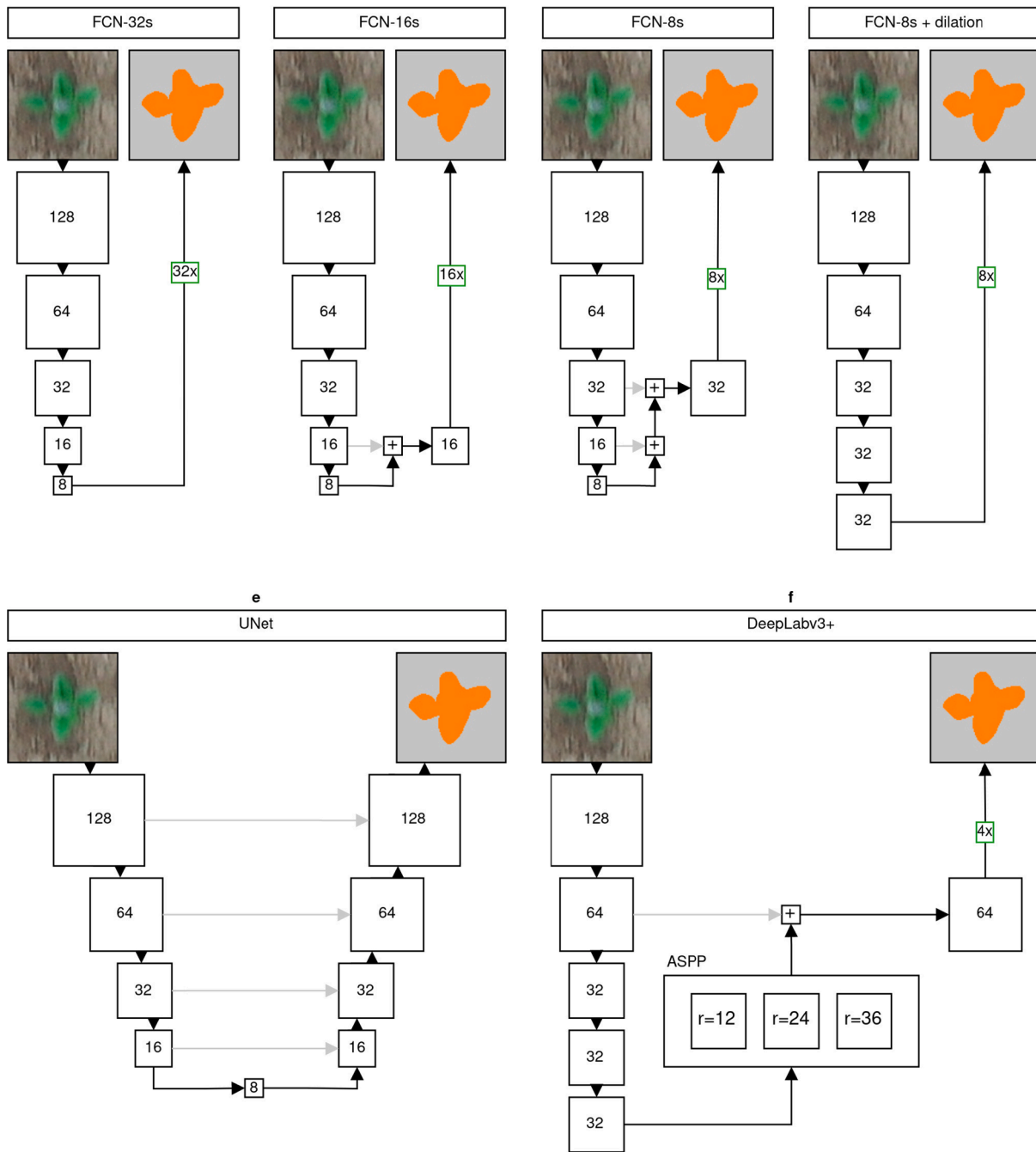
Fig. 2. Model diagrams of the different semantic segmentation architectures used in this study. Numbers indicate the spatial resolution of the feature maps. Skip connections are shown as gray arrows. The concatenation of feature maps is shown as plus. Upsampling operations before the concatenation is omitted for readability. Final bilinear interpolation is shown in a green box indicating the upsampling factor. a-c Modifications of the FCN architecture with different strides. d FCN architecture using dilated convolutions, preserving the spatial resolution in the last layers. e UNet architecture using skip connections. f DeepLabv3+ architecture using Atrous Spatial Pyramid Pooling (ASPP) with atrous rates of r = 12, 24 and 36 .
