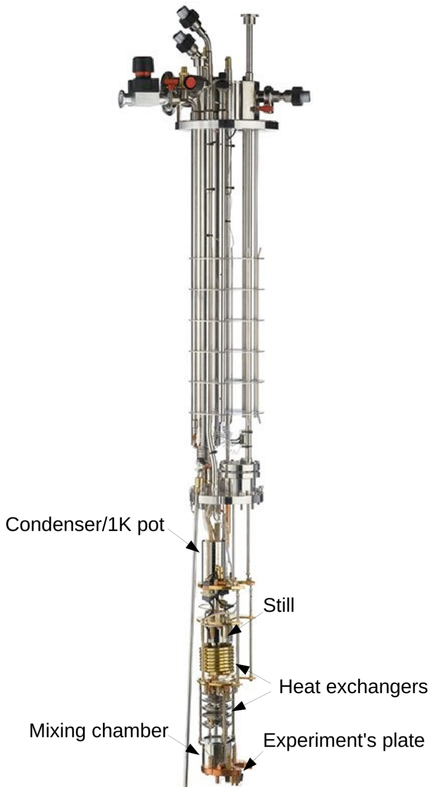
Figure C.2: This picture corresponds to the cryostat OXFORD Kelvinox100 used for the experiments performed at the TUM.
