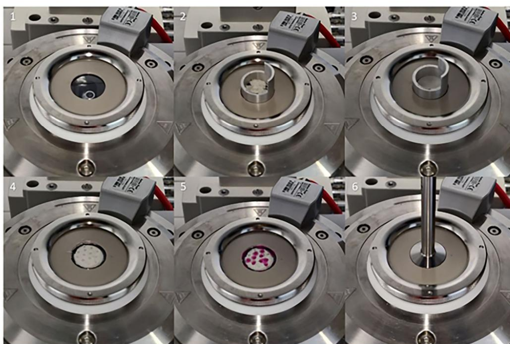
FIGURE 2 Setup of the coupling between rheometer and confocal laser scanning microscope. Process of sampling and setting the upper rheometer geometry with flour S3.
