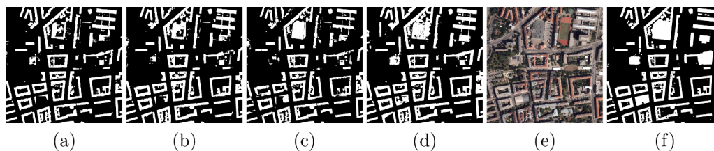
Fig. 11. Examples of building extraction results obtained by different learning methods. (a) Baseline-t. (b) Baseline-a. (c) Baseline-a+t. (d) CrossGeoNet. (e) and (f) are INRIA aerial imagery and ground reference from Vienna. Auxiliary and target sets are chosen from Vienna for ensuring similar data distribution.
