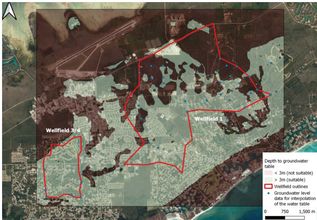
Figure 4. MAR suitability map with respect to the depth to the groundwater table for the populated areas of wellfields 1, 3, and 4 (source of base map: © Google Maps).
