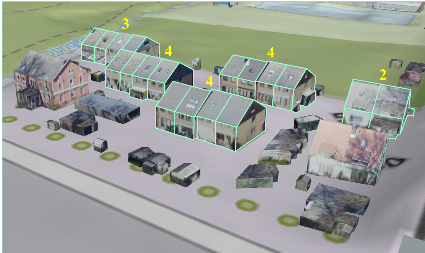
Figure 7.16.: A 3D view of building split changes of an excerpt area (Kieler Straße) from the Hamburg datasets based on Figure 7.15. The buildings shown have been split into between two and four smaller adjacent buildings (yellow texts and cyan wireframes). Source: Landesbetrieb Geoinformation und Vermessung Hamburg, 2024.
