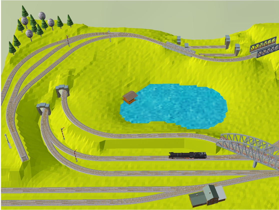
Figure 3.10.: Visualization of a segment from the Railway-Scene dataset (Häfele & Nagel, 2015) using the 3DCityDB Web Map Client (Yao et al., 2018). The dataset, presented in LOD3, incorporates various city objects from all fourteen thematic modules in CityGML (Gröger et al., 2012): Core , Appearance , Building , Bridge , Relief , CityFurniture , Generics , CityObjectGroup , LandUse , TexturedSurface (deprecated), Transportation , Tunnel , Vegetation , and WaterBody .
