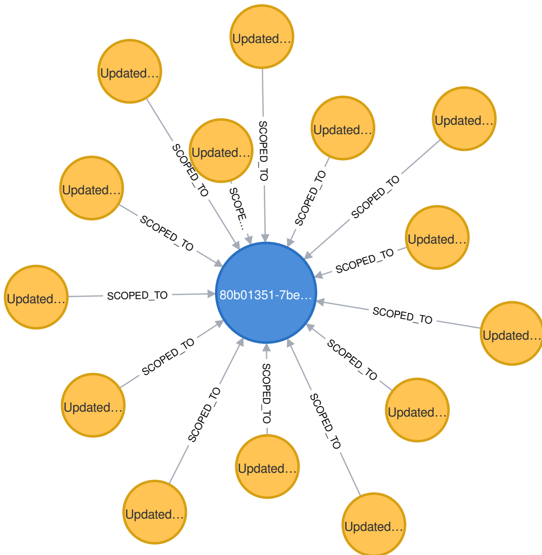
Figure 7.21.: Visualization of scope nodes (orange) representing all 14 clusters of buildings. In each cluster, all buildings share the same updated creationDate value. The information stored in each scope node includes the number of buildings that share the same updated property value, the cumulative bounding box containing all these buildings, as well as additional spatial indicators such as the spatial and type coverage of the current cluster over the entire city model. These scope nodes are attached to the city model node (blue). Visualized with Neo4j Browser.
