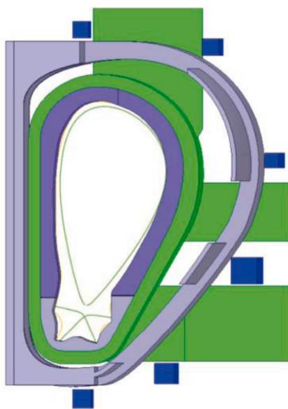
Fig. 14. Conceptual in-vessel segmentation for the SF divertor [8]. There is space for a horizontal port between the PF coils, although insufficient clearance for the proposed cassette.
