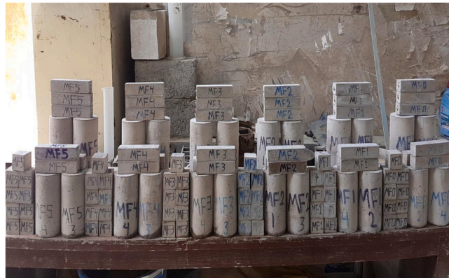
Fig. 8. Curing of the specimens.
