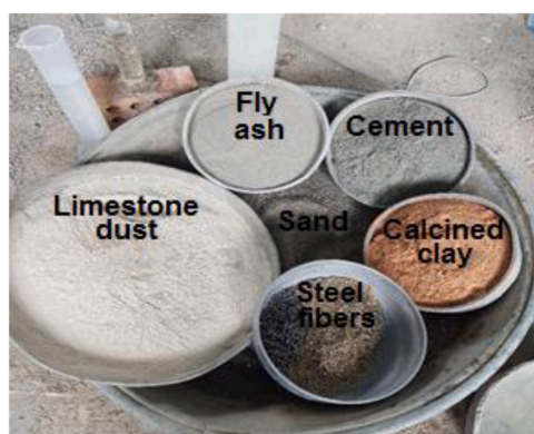
Fig. 6. Ingredients of the produced green mortar.
