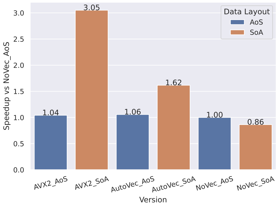
Figure 3.12: Speedup of iteratePairwise() from vectorization for the Linked Cells container. A handwritten intrinsics functor achieves significantly better performance than the auto vectorization by the Clang 17 compiler. For details about the setup see Section A.1.2.
