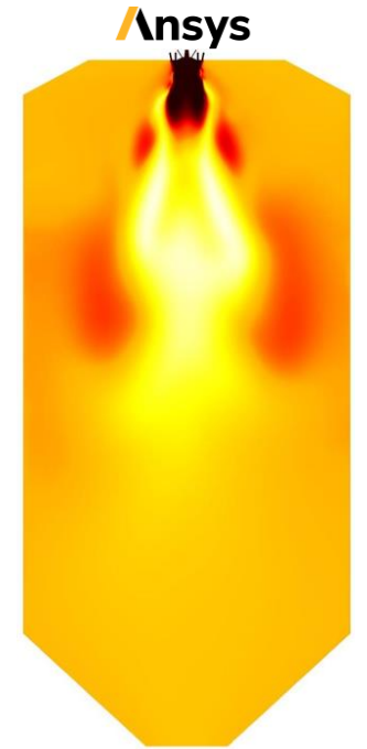
Session 10-5: CFD modeling of allothermal plasma-assisted entrained flow gasification (Sebastian Wilhelm, TU Munich)
