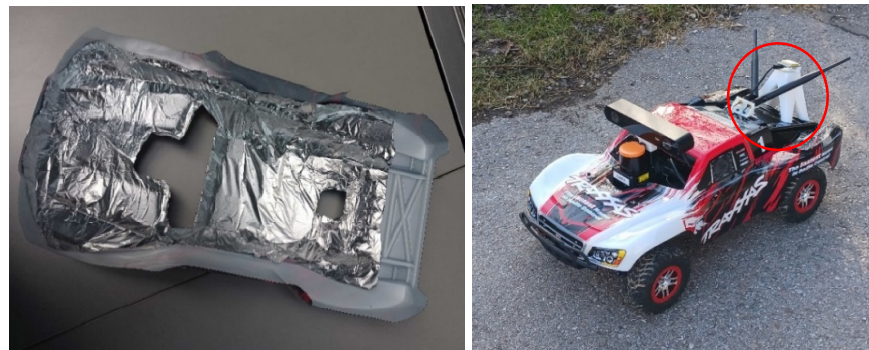
Figure 3.12: On the left: aluminum shielding applied to the inside of the vehicle's hull before installation of the grounding wire. On the right, the final mounting position of the GPS receiver at the rear of the vehicle on its standoff (red circle).
