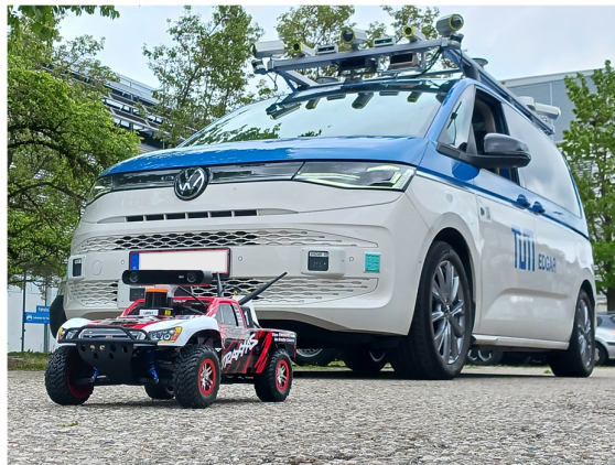
Figure 5.3: The F1TENTH-platform-based vehicle developed in this thesis in front of the TUM's EDGAR vehicle which Appendix C presents.
