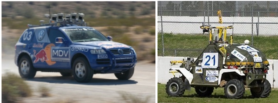
Figure 2.2: Different (and similar) approaches to Offroad Autonomous Driving. On the left, Stanley of Stanford University [14], and on the right AVIDOR-2004 of Team SciAutonics [16].
