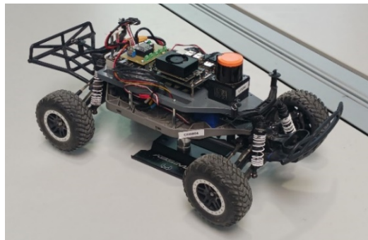
Figure 3.3: Initial configuration of the F1TENTH platform supplied by TUM’s AVS department.
