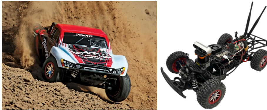
Figure 2.6: On the left, a stock Traxxas Slash 4x4 model driving in its intended environment [31], on the right an example finished configuration of an F1TENTH vehicle based on the Slash chassis and drivetrain [32].
