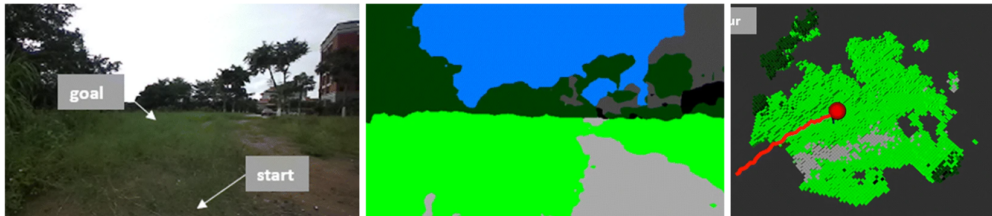
Figure 2.13: RSPMP perception pipeline, left, example RGB camera input, middle, semantic segmentation results for that image, right, 2D-projected result map containing semantic segmentation results.
