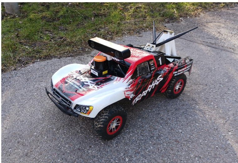
Figure 6.1: Final version of the modified F1TENTH platform developed in this thesis.
