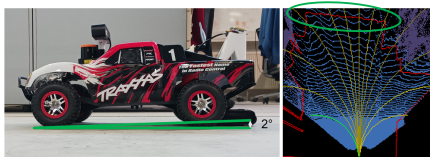
Figure 4.5: Left, the minimum tilt forward to cause a ground strike (barely visible in the tires as the suspension is drooping). Right, a top-down map (Section 3.3.2) with a ground-strike in the LiDAR data, were the ground-strike-related data points in the green circle.
