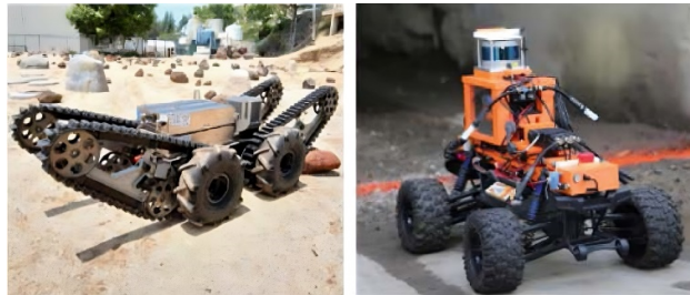
Figure 2.4: Robots for extreme off-road terrain: left 'Tracked', and right 'Ackermann', which [26] tests and evaluates in tunnels and mines.
