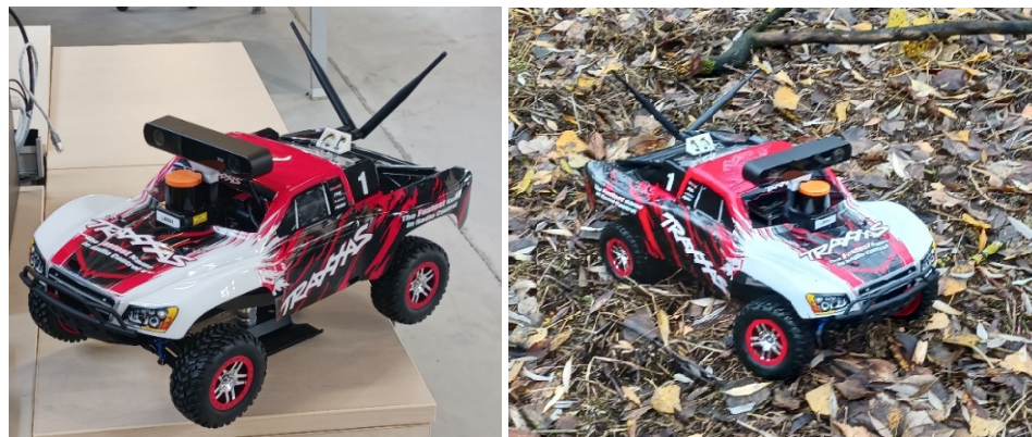
Figure 3.5: Modifications of the provided F1TENTH platform vehicle. Left, modifications with plastic outer shell. Right, data gathering run in off-road environment.
