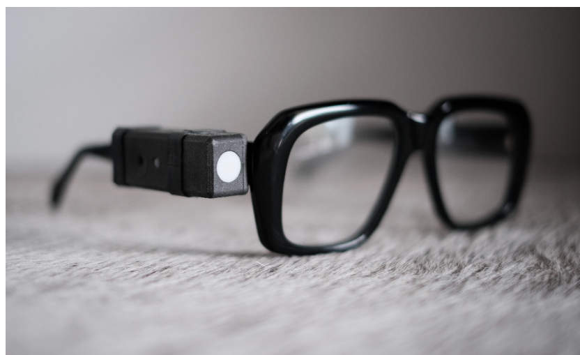
Figure 7. The wearable light dosimeter, “lido”, attached to a pair of glasses. The white circle is the diffuser. The small grey circle on the left is an indicator light that flashes green every 10 s (0.1 Hz) when recording.
