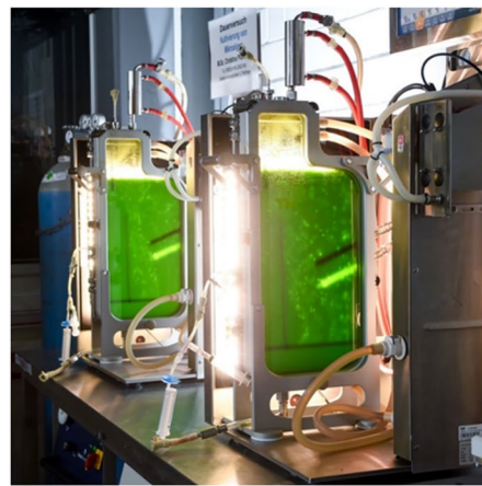
Flat-plate gas-lift reactor (0.1 m 2 )
