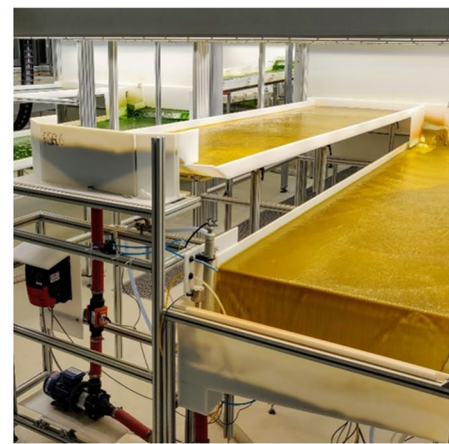
Open thin-layer cascade reactor (8 m 2 )
