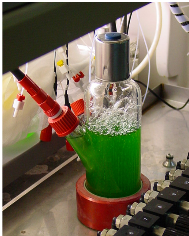
Fig. 2 Bubble column photobioreactor with 200 mL working volume, defined gas flow and pH electrode in an illuminated incubator [109]
