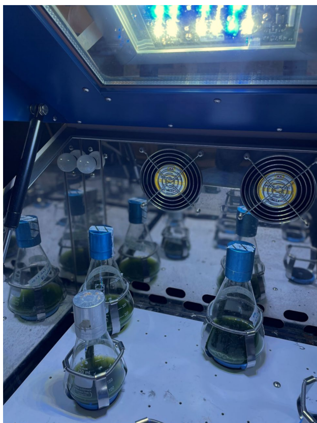
Fig. 1 Shake flasks with 50–100 mL microalgae suspension inside a shaking incubator. A LED-panel is placed on top of the transparent incubator cover. An alternative is the individual illumination of shake flasks from the bottom up by individual LED-panels (not shown)
