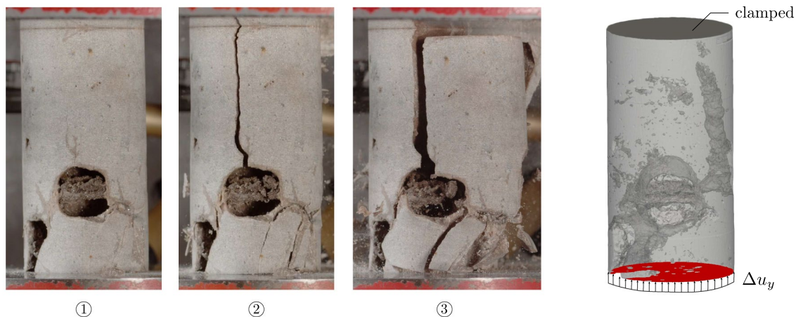
Fig. 9 Experimental setup and recorded crack pattern (left), and simulation setup (right) based on the CT-scanned drill core
