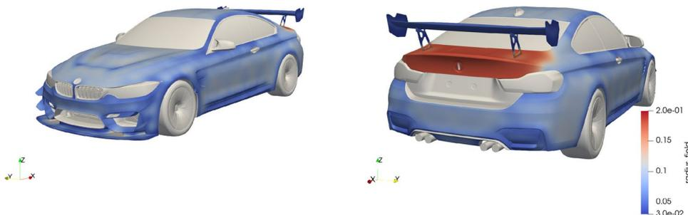
**Fig. 16** Geometrical constraint: constrained zone—red, free design surface—blue, non-design parts—light gray
