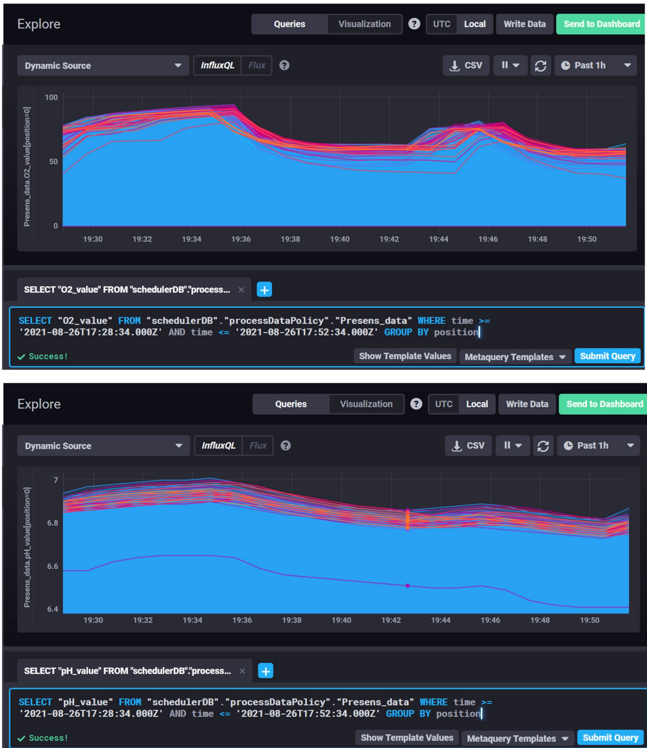
Fig. 4 The browser-based graphical user interface Chronograf connects to the InfluxDB and allows for real-time data visualization. In this figure, the process parameters dissolved oxygen (top) and pH
