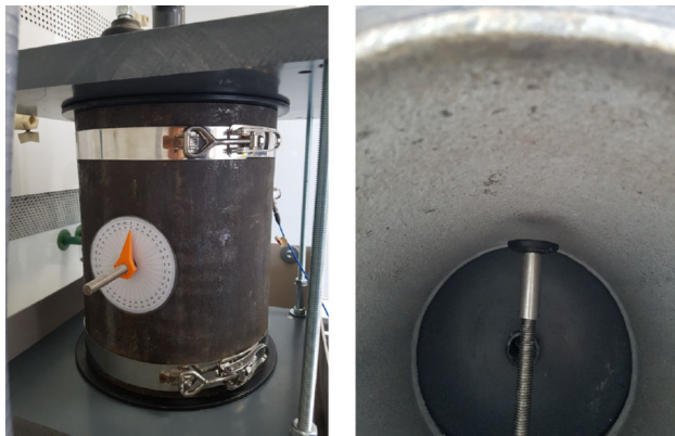
Fig. 3 Mechanical measurement of scaling thickness: The threaded rod is rotated until the rubber tip hits the scaling surface. The relative change in the number of rotations is recorded at each time interval
