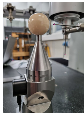
Fig. 3 Reference sphere with temperature sensor for measuring tip calibration
