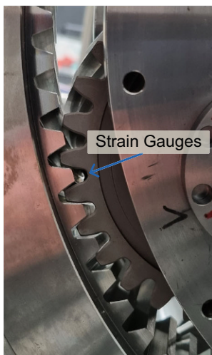
Fig. 2 Loaded gear teeth of planet and ring gear mesh
