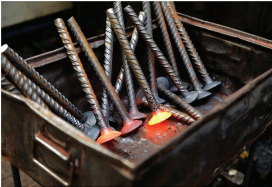
Figure 3: PSB® Headed bars manufactured by hot forging
