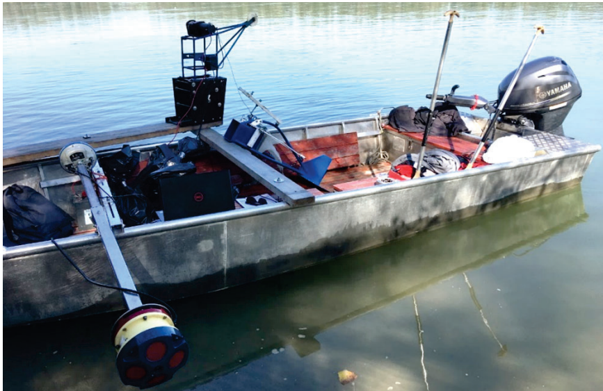
Figure 8: Additional site measurements - ADCP instrument (left) fixed to the BME's measurement vessel – © BME / CÉH
