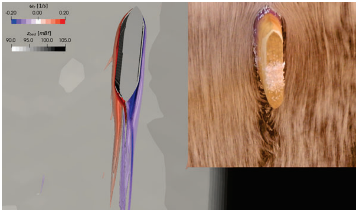
Figure 10: Comparison of small-scale test and CFD model results in the vicinity of the left bank pier (design variant 2), river flow to be considered from the top to the bottom – © BME / CÉH
