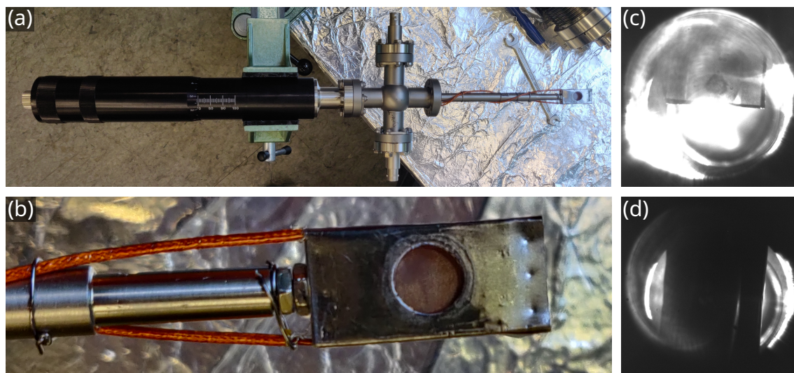
Figure 4.3: Photos of the single-electrode Faraday cup. (a) Top view of the full assembly with the Faraday cup mounted at the end of a linear transfer that is connected to a four-way CF-16 cross together with two BNC feedthroughs. (b) Magnified view of the Faraday cup. (c) + (d) Backside of the Faraday cup inside the cluster source taken from the preparation chamber through a lens stack with the position of the linear transfer at (c) 62 mm and (d) 75 mm.
