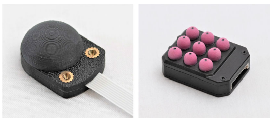
Fig. 9 Left: Single 3D force tactile sensor. Right: A slim tactile sensor array (PapillArray Sensor) available in different configurations. Images from Contactile https://contactile.com/ licensed under CC BY-NC-ND 4.0
