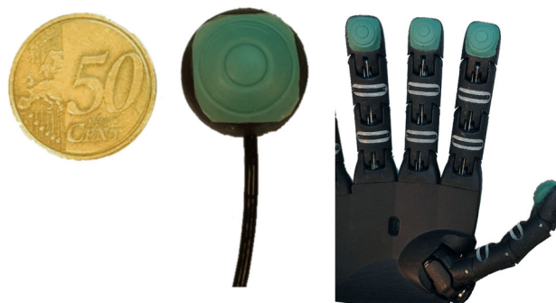
Fig. 7 Left: the SINGLEX stand-alone tactile pressure sensor version. Right: FTS tactile pressure sensor mounted on a robot finger. Images used with permission from Seed Robotics https://www.seedrobotics.com/
