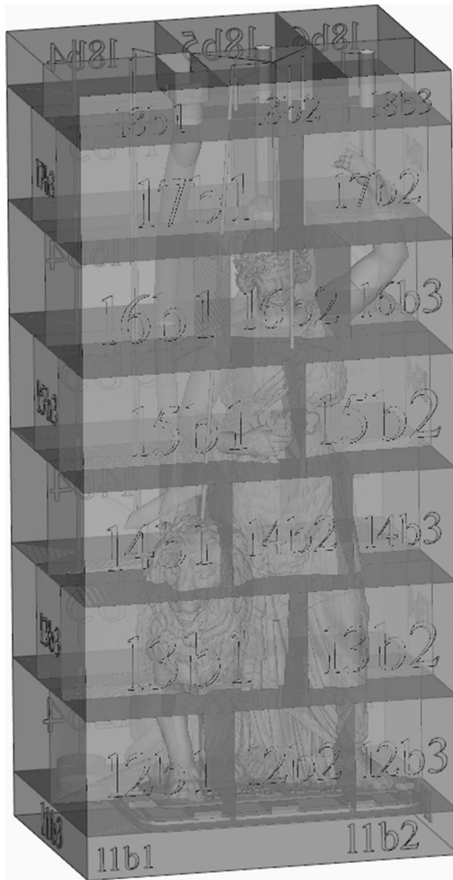
Figure 10. Stack-mold design of a complex 48 parts core package (left). The cast part is characterized by many freeform surfaces and undercuts (right).
