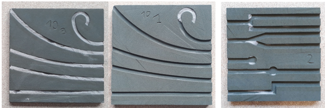
Figure 6. Specimens for cleaning tests, opened for examination—continuous shapes (left) and unsteady changes in cross section (right).
