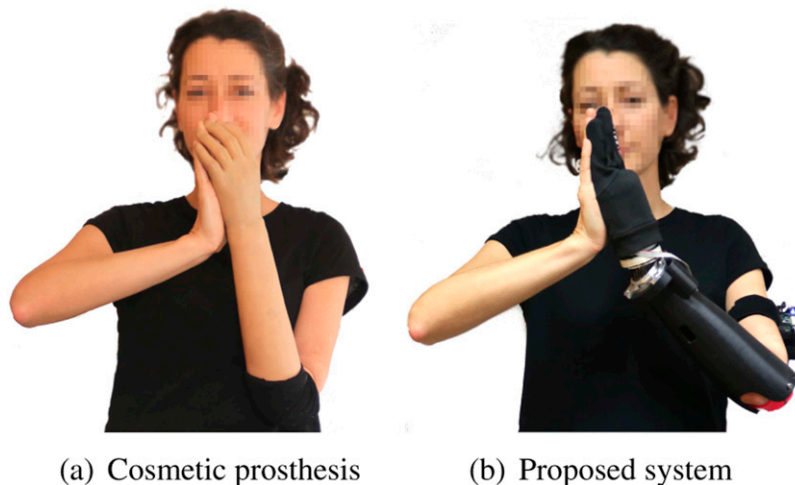
Figure 2. Prosthesis user wearing (a) her own esthetic prosthesis and (b) the proposed 3 DoFs wrist system.
