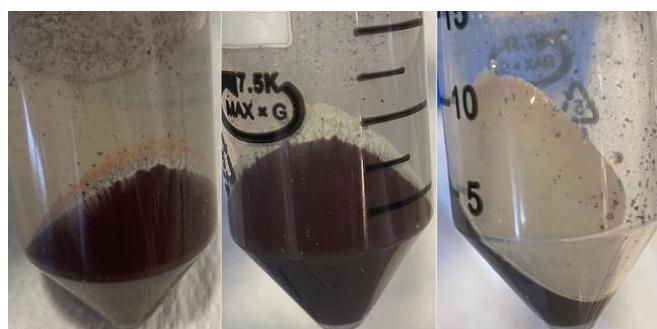
Figure 2-7. The centrifugation technique separates the activated catalyst slurry from the reaction mixture in a centrifuge tube after the activation step of the two-step Reppe ethynylation process. The liquid layer supernatant solution is decanted, while the solid layer catalyst slurry is retained (left). It is then washed and purified using the same methods. However, the retained catalyst slurry after centrifugation contains a relatively large amount of moisture. It may reduce the purity of the catalyst. Additionally, the centrifugation force may also potentially destroy the catalyst's metal-support structure, which causes the leaching of active species (dark brownish residue at the bottom) from the supporting material (white species on the top layer at the surface of the interface).
