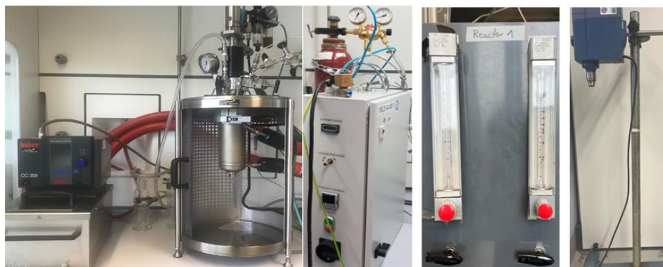
Figure 7-1. The photos of some proposed test units and accessories for the catalytic ethynylation process. The trial-tested autoclave reactor was equipped with a digital temperature controller and a pneumatic agitator for the catalytic performance test of Reppe ethynylation (left). The rotameters control the acetylene gas flow rate (middle). The overhead mechanical stirrer to agitate the reaction mixture (right).
