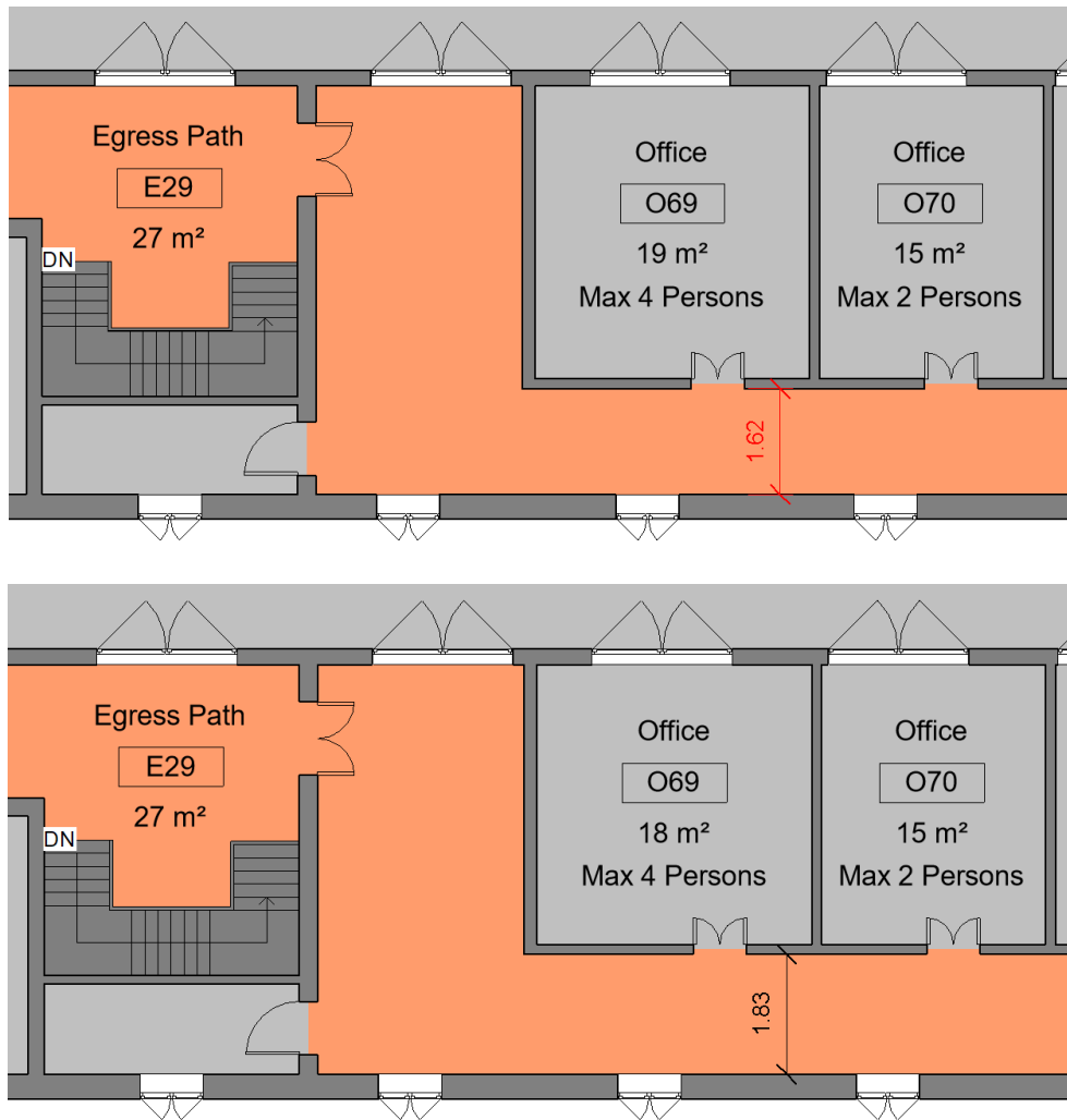
Figure 5.6: Adjusting the width of the side corridor according to the IBC standards
