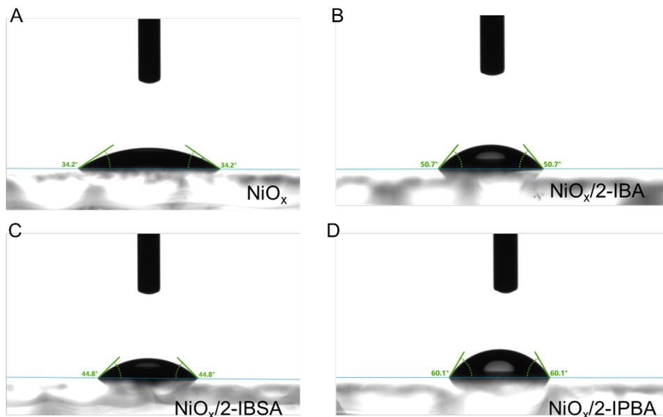
**Figure 5.5:** Contact angle testing for (A) the  $\text{NiO}_x$ , (B)  $\text{NiO}_x/2\text{-IBA}$ , (C)  $\text{NiO}_x/2\text{-IBSA}$ , and (D)  $\text{NiO}_x/2\text{-IPBA}$  substrates. Reproduced from Ref. [67] with permission. Copyright 2023, Royal Chemistry of Society.
