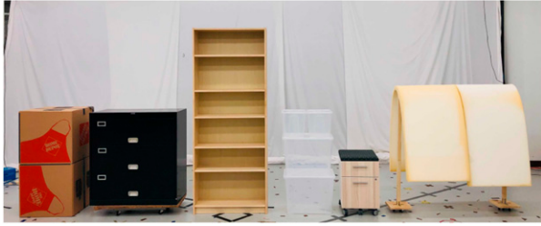
Figure 7. Obstacles used in the NLOS tests. The materials of the obstacle from left to right are cardboard, metal, wood, plastic, wood, and foam.
