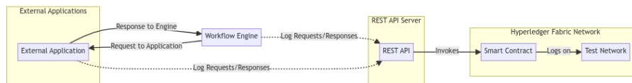
Fig. 2: Architecture of the REST API-based approach. The workflow engine initiates a process that interacts with external applications and logs these interactions through the REST API to a smart contract deployed on the Hyperledger Fabric network.
